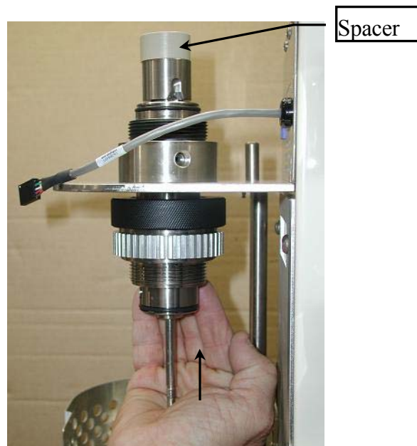
Figure 3-4 Bob Shaft Removal
